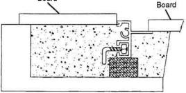
Be very careful that the concrete is absolutely smooth and level with the inside lip of the frame. This will allow the mat to lie perfectly flat and avoid rocking.
