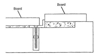
Be very careful that the concrete is absolutely smooth and level with the inside lip of the frame. This will allow the mat to lie perfectly flat and avoid rocking.
