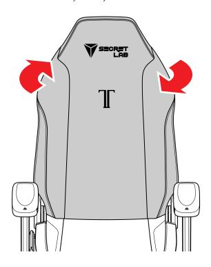
**04** While holding the backrest in position, fully tighten the M8 screws on the **LEFT** side. You may have to push the left side of the backrest in the direction as shown above, until the desired alignment is achieved.
