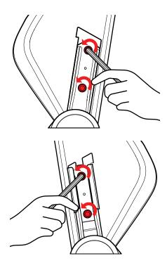
Adjust the backrest until it is aligned, then hold it in position. While still holding the backrest in position, use the allen key to fully tighten the M8 screws on the **RIGHT** side first.
