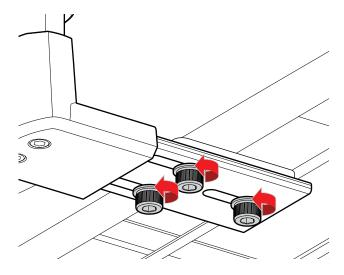
O3 Slide the metal plate to adjust the armrest width inwards or outwards. Adjust the armrests based on how they look in relation to the chair, instead of the position of the metal plates underneath.
