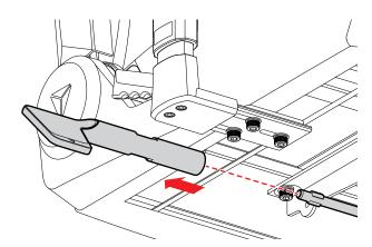
**02** Loosen the three M8 screws using the allen key provided.
