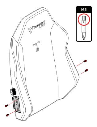
Push the left recline bracket up to align with the screw holes on the left of the backrest. Insert the M8 screws and fully tighten all 4 screws on both sides with the long allen key.
