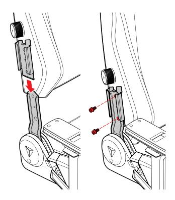
1 Install the magnetic side covers by aligning them on top of the backrest brackets on both sides. They will magnetically snap into place.
