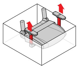
Place the wheelbase upside down on top of the foam sheet and insert all 5 casters.
