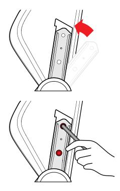
Slide the backrest bracket on the right down onto the right recline bracket until it comes to a stop. Insert the M8 screws (from Step 4) and screw them in halfway.
