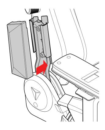
Remove the recline strap. Next, use the Phillips screwdriver to remove the red screw marked out by the red safety tab on the right recline cover.
