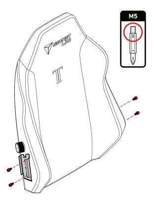
Push the left recline bracket up to align with the screw holes on the left of the backrest. Insert the M8 screws and fully tighten all 4 screws on both sides with the long allen key.
