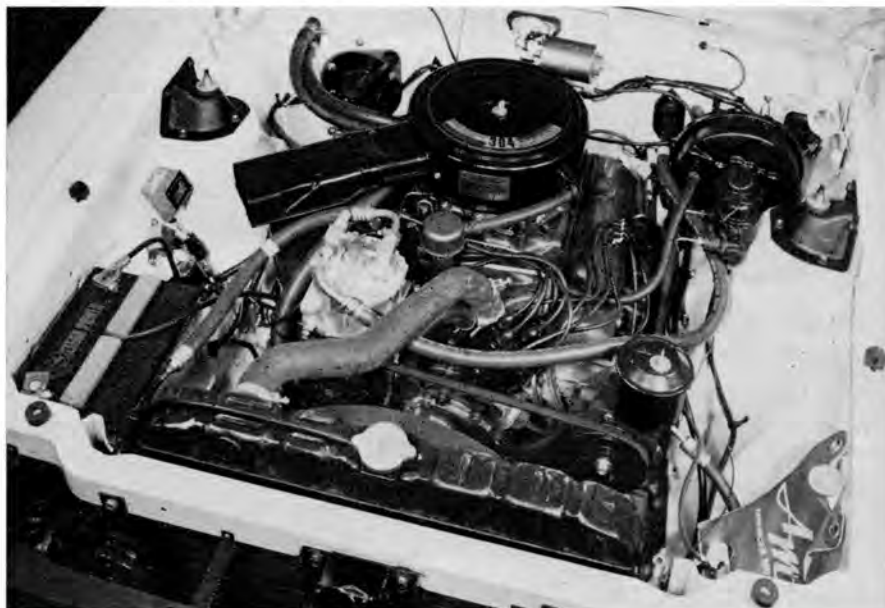
304-CID V-8 is top of the line, produces 210 bhp using 9:1 compression ratio and two-barrel carb; 199 and 232 sizes are also offered.
