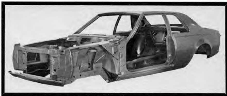
UNIT BODY/FRAME, by now a tradition with AMC, is used for Hornet. Though not yet offered, body could accept either big AMC engine.
