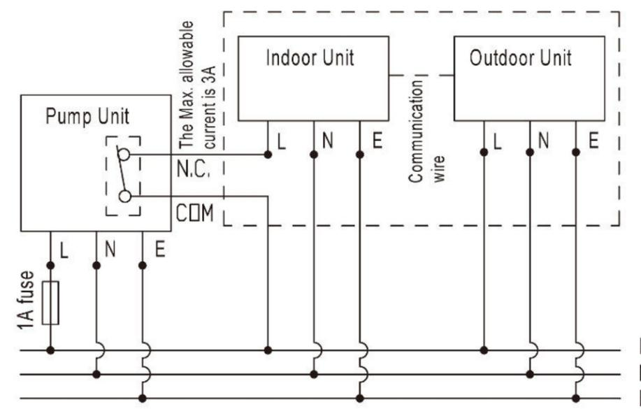
1. Please refer to the wiring diagram of the air conditioner manufacturer within the dashed box.
