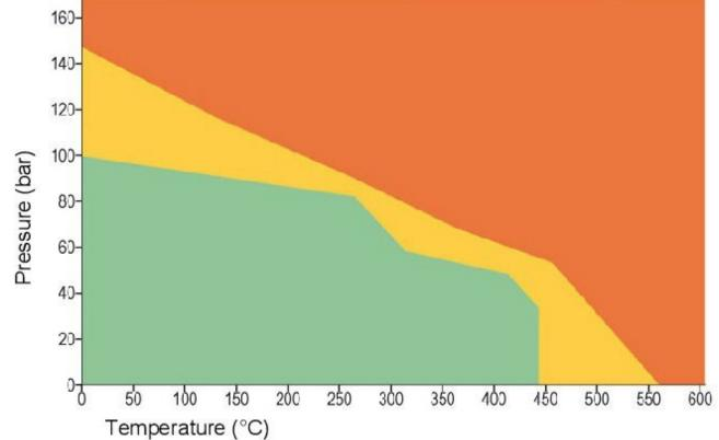
The P x T diagram above indicates the service limits for NA-1122 considering the simultaneous influence of pressure and temperature (chemical suitability assumed). The green area represents the normal service limits, for the yellow area consultation is recommended, while the orange colored area shows the maximum application limits for which technical consultation is mandatory.
