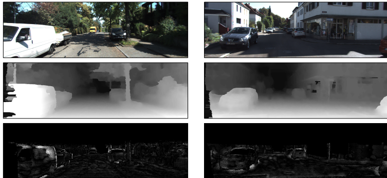
Figure 2.8: Example results from the KITTI dataset. Top to bottom: left image, disparity map, and clamped disparity errors.
