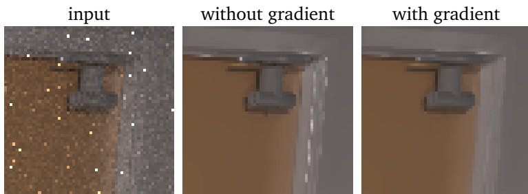
Figure 8.4: Filtered output for the “conference” scene without (middle image) and with the feature gradient (right image). Including the gradient term improves filtering along edges.
