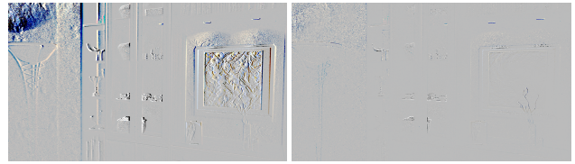
Figure 9: Temporal differences with motion vectors. Left: Motion unaware temporal differences in a frame of the BOOKSHELF sequence at 512 samples per pixel. Right: Motion aware temporal differences for the same setup. The motion-aware temporal differences on the right are significantly smaller (gray represents zero).
