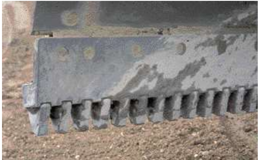
The carbide-tipped bits on a cutting edge can be a valuable tool in preparing a road for Chloride treatment. They penetrate the road and give a shallow scarifying effect to loosen and mix the existing gravel. This leaves a nice uniform loose layer of material on the surface.
