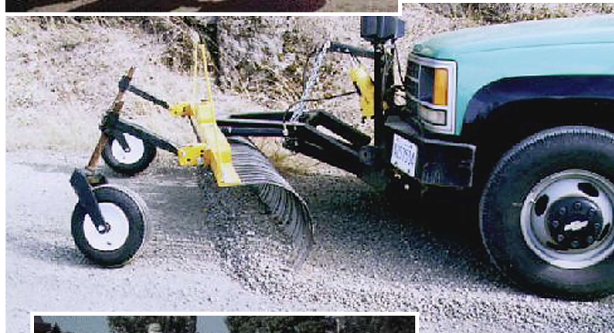
A simple front-mounted rake attachment for a pickup truck. The vehicle can be used daily for other work such as sign maintenance, either while using the rake or after the rake has been removed.
