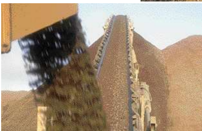
The discharge conveyor from a crushing plant is in the foreground. Notice how badly segregated the material is as it is carried up to the stockpile on a belt stacker. This invariably leads to problems illustrated in the following two photos.
