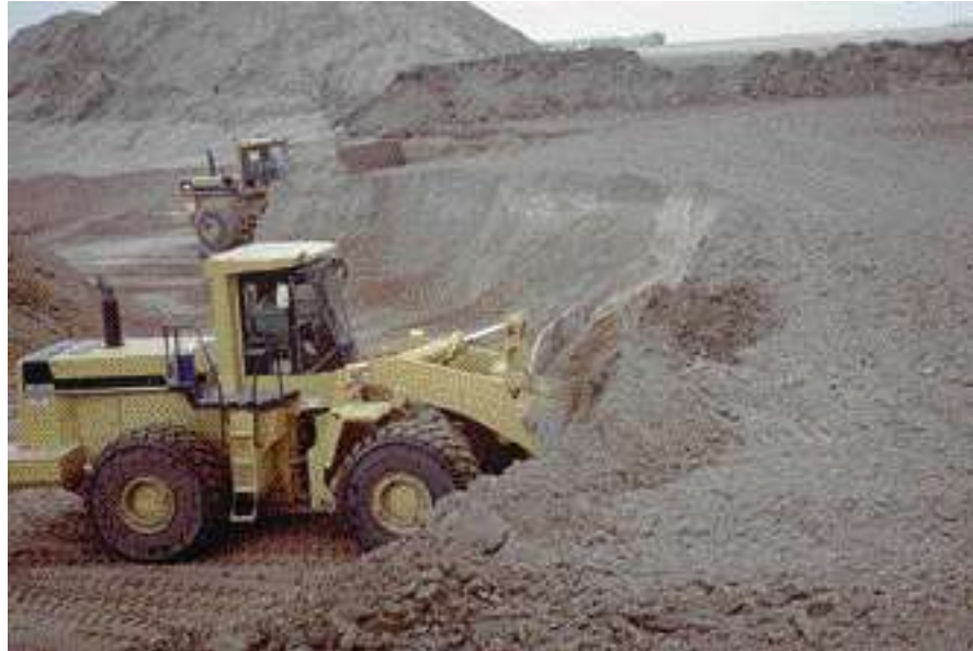
A very good example of working a gravel bank. Large loaders are being used to feed a crushing plant. Notice the good effort to work a broad area of the gravel bank. The operator virtually never takes a bucket of material from the same spot twice. This assures a good blend of material going into the crusher.
