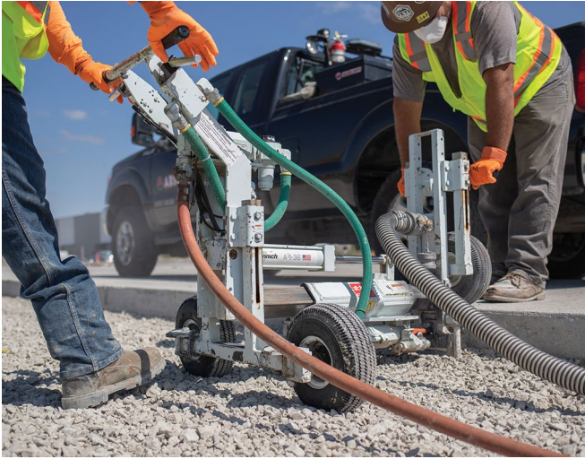
Figure 38. Small grade-reference drill rig
