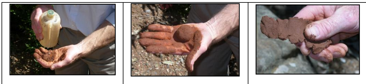
Figure 3. Hand texturing soil samples in the field
