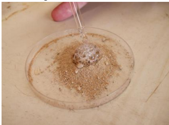
Figure 7. “Fizz” test for carbonates. .
