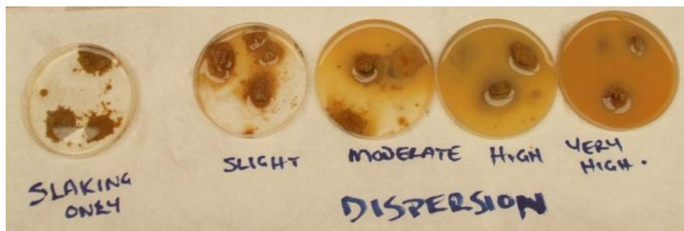
Figure 1. Field dispersion of a number of clay samples
