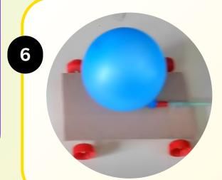
Blow into the straw to inflate the balloon, then pinch the end to hold the air. Let go and watch your car zoom forward as the balloon deflates!
