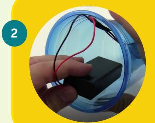
Connect the motor's wires to a coin battery, making sure the connections are tight and secure.
