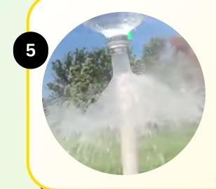
When the pressure is high enough, the cork will pop, and the water bottle rocket will launch into the air!
