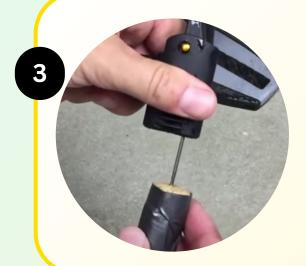
Attach a bicycle pump with a needle nozzle to the cork.
