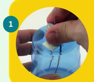
Attach the small motor to the bottom of a lightweight cup using tape.
