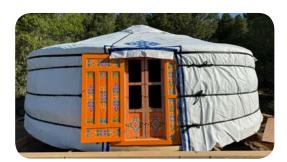
Diameter: 21 to 22 feet (6.6m) Wall height: 5 feet (1.6m) Height in center: 8 feet (2.45m) Dimensions may vary slightly.
