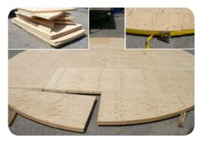
**SIP with Protective Treatments:** On request, we can also apply a weather treatment to the bottom side of the platform and a varnish to the top side. The bottom-side treatment is an application of Thompson Water Seal. For the top side treatment, we apply two layers of high-quality latex varnish. Our available varnish colors are Danish Walnut (dark brown) or Juniper Ash (light grey)
