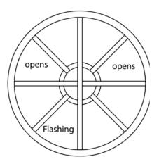
The full acrylic *toono* can also be fitted with a chimney flashing for stove pipe passage. Check out our Full Acrylic *Toono* Finish video here:
