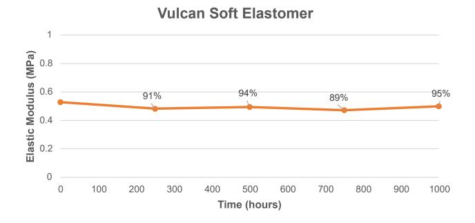
ASTM G154: Cycle 1 ASTM D412: Die C, 500 mm/min, average values represented.
