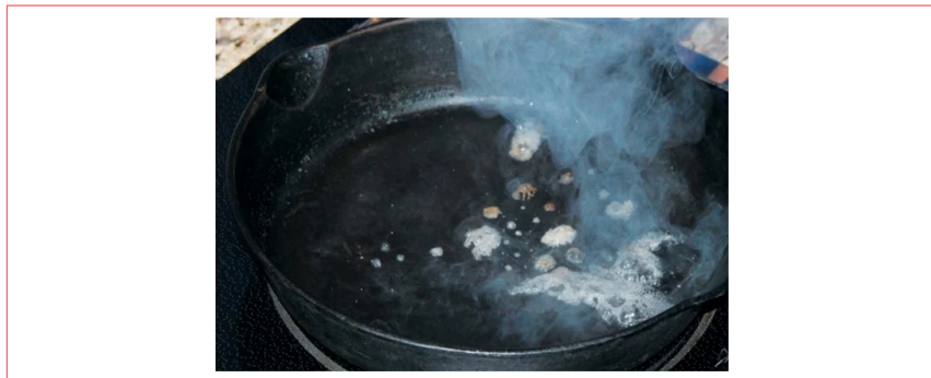
FIGURE 2: Result of about 1 teaspoon of water being added to a cast iron skillet. Full evaporation required approximately 10 s. Note that some droplets are colored due to contamination on the skillet surface. Reprinted from reference (4) with permission of the author.
