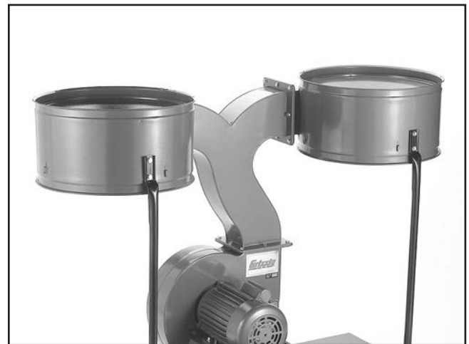
Figure 18. Collectors installed (G0562Z shown).
