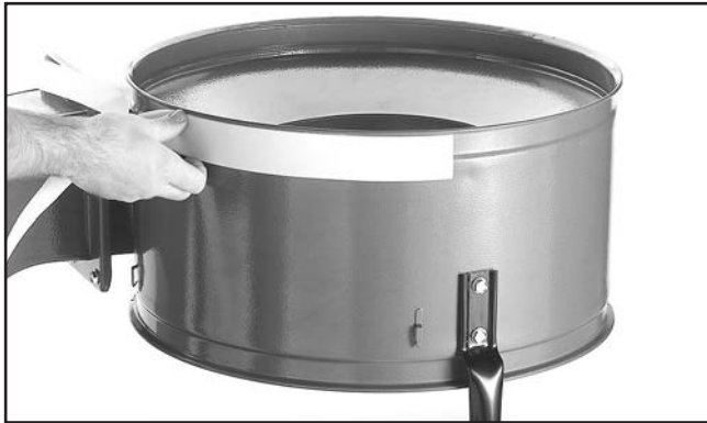
Figure 19. Installing wide foam strip.
