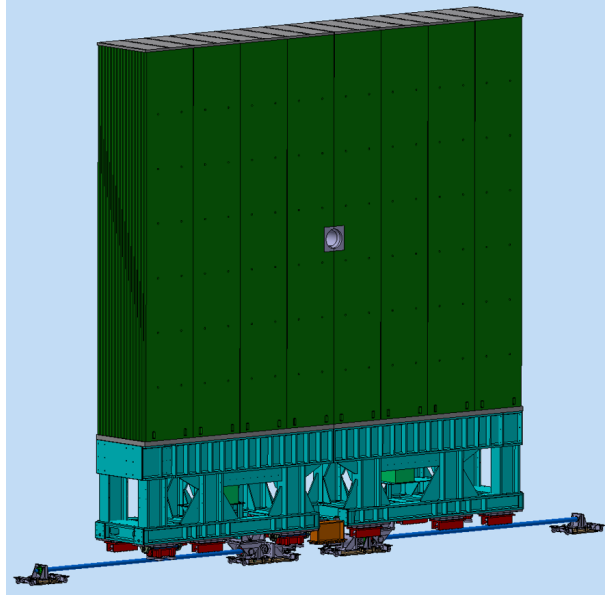
Figure 5.9: A possible design of the new muon filter, making use of the iron slabs from the OPERA magnet.
