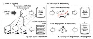
Fig. 1. A simple generalized view of the partitioning process.
