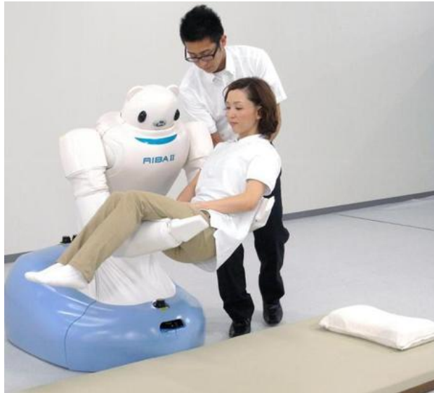
Fig.1 RIBA-II 1/2 , a “caregiving” robot able to lift and carry patients up to 80kg of weight (Source: Riken Research Center, 2011).
