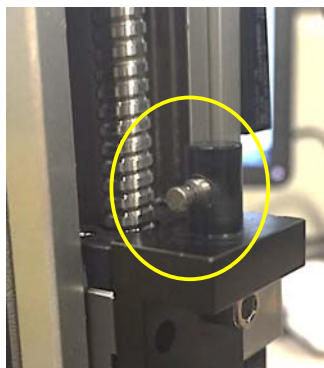
Figure 8. Clearance between dowel pin and the external shaft connected to the U-joint.
