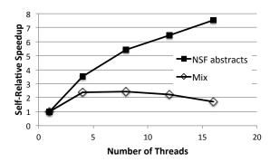
Figure 1: Self-relative performance scalability of the K-Means operator.
