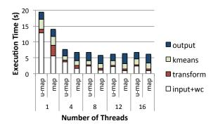
Figure 4: Execution time of the TF/IDF-K-Means workflow on the *Mix* input using a std::unordered\_map (u-map) or a std::map.
