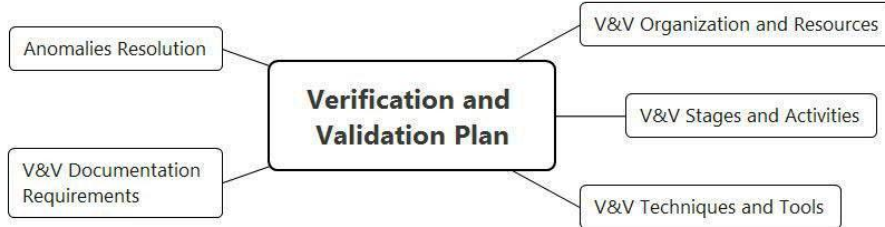
Fig. 9. A structure of V&V Plan complied with IEC 61508-2 (Section 7.1)
