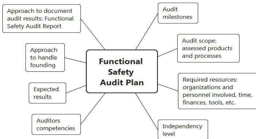
Fig. 12. A structure of Functional Safety Audit Plan complied with IEC 61508-1 (Section 8)
