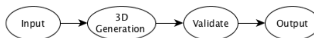
Fig. 1. The abstract layer of a workflow. Vertices represent tasks, edges indicate the execution order. At this point, no implementation or technical details are represented.
