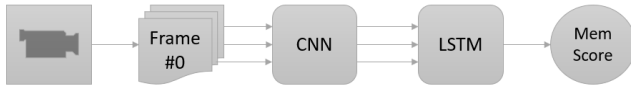
Figure 1: The proposed method for predicting memorability scores of videos using deep features and LSTM.
