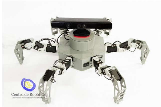
Figure 1. CRABOT, a six-legged 3D-printed platform designed for exploration and object manipulation. Platform features are listed in table 1.
