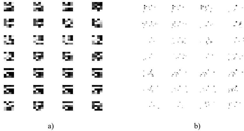
Fig. 5. Matrix of DTW pair correlation for samples of different facial expressions without thinning - a) and two-dimensional thinning using DCT - b).
