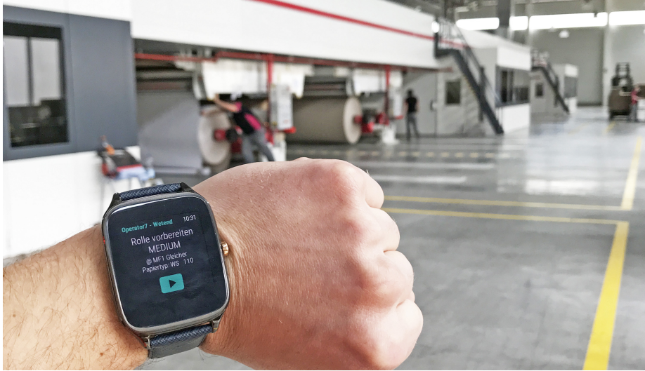
Fig. 5: Exemplary process based user interface in corrugation plant
