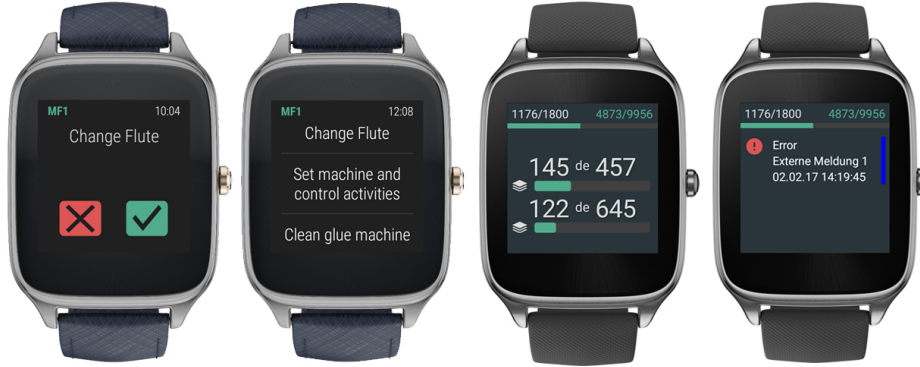
Fig. 3: Wearables: a) unclaim/complete task; b) tasks; c) and d) context info
