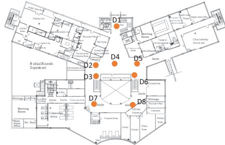
Fig. 7. Lbeacons on 2F of OM Building
