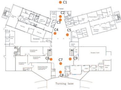
Fig. 6. Lbeacons on 1F of OM Building
