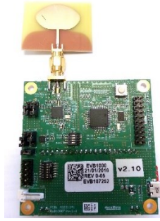
Fig. 4. Decawave EVB1000 individual module, used for both fixed beacons and mobile nodes.
