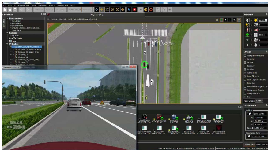
Figure 8: SCANer test environment
