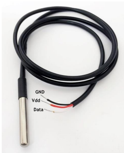
Figure 5. Waterproof temperature sensor DS18B20.
