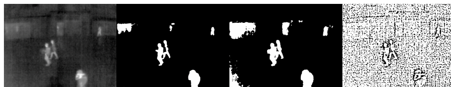
(a) Original segmen- (b) Global Thresh- (c) Otsu Threshold- (d) Adaptive Mean tation olding (t=80) ing Thresholding
