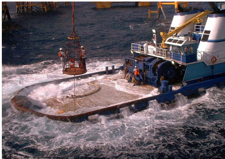
Fig. 3. Lowering the basket with the turn at the Pivot Point
