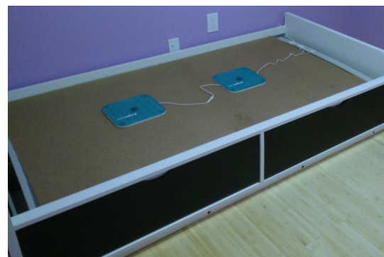
Figure3: Sensor for movement detection on the bed under the mattress
