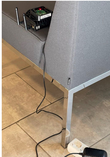
Figure 9: One of the base stations including both WiFi and UWB anchors
