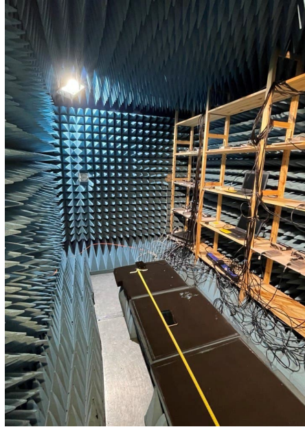
Figure 4: Collecting WiFi RTT measurements inside the Anechoic Chamber
