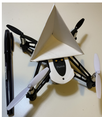
Figure 3: Parrot Mambo Minidrone, with a trihedral retroreflector to increase mmWave detectability.
