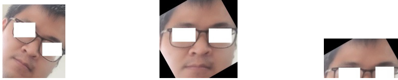
Figure 2: Utilizing key points to rotate and crop the facial image
