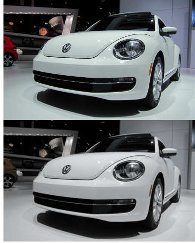
Figure 5: A positive blurred image test performed with EfficientNetB5. The upper image is the original one, yet misclassified as a sports car. The bottom one was blurred via a Gaussian kernel with a standard deviation of 1.5 and correctly classified as a hatchback.
