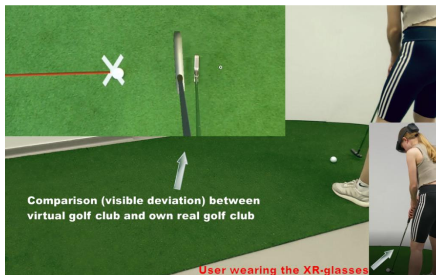
Figure 1: Illustration of the XR golf putt training. The upper left image shows the user's view through the XR-glasses, including the visible deviation of the user's own club guidance (on the righthand side) from the virtual golf club (on the left next to it) as well as the virtual red line guiding the direction from
