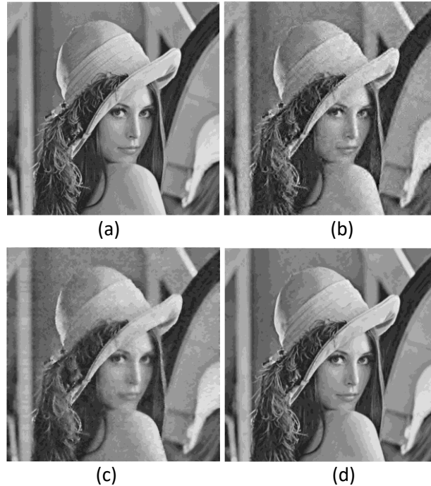
Figure 4. Reconstructed Lena under compression rate with 0.25. (a) the original image; (b) PCS-RP (26.84 dB); (c) PCS-RP (26.78 dB); and (d) our method (PSNR= 34.98 dB).
