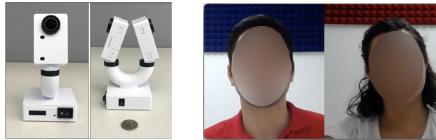
Figure 1: Left: The device used to record the conversation. The device has two cameras, each pointing to one party of the conversation. Right: Example of videos shown to the human raters. The video contains synchronized videos of the heads/faces of both the participant and the confederate as recorded by the device on the left. The video of the participant's face only served as input to the AI pipeline.
