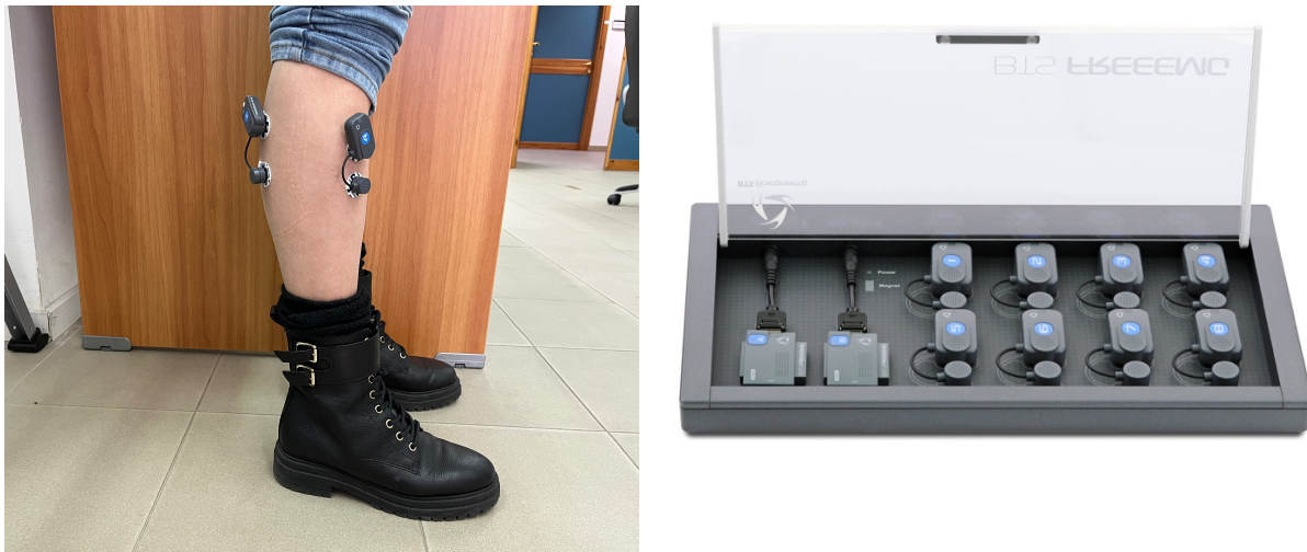
Figure 1: Positioning of the electrodes on Gastrocnemius Lateralis and Tibialis Anterior muscles and used platform.
