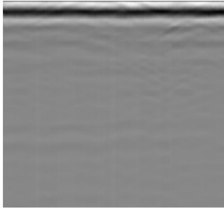
Figure 2: GPR scan of the soil layer without mines
