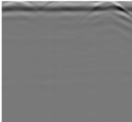
Figure 3: GPR scan of the layer of soil with mines
