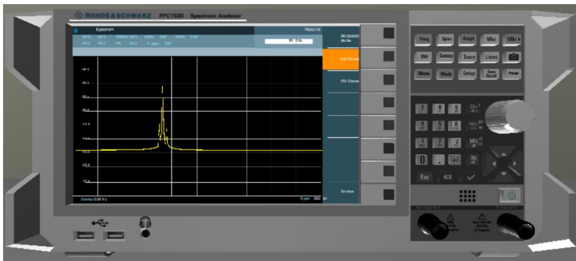
Figure 4: AM signal spectrum on the spectrum analyzer model screen
