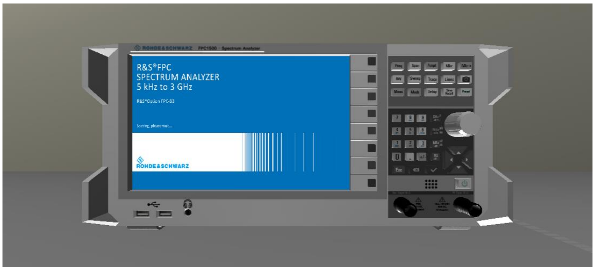
Figure 3: Computer model of the FPC1500 spectrum analyzer
