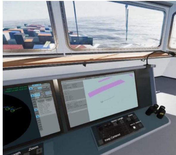
Figure 2: The important keys of the radar and ECDIS are modeled on top of the keyboard to improve the usability of presses that require finger fine motor skills.
