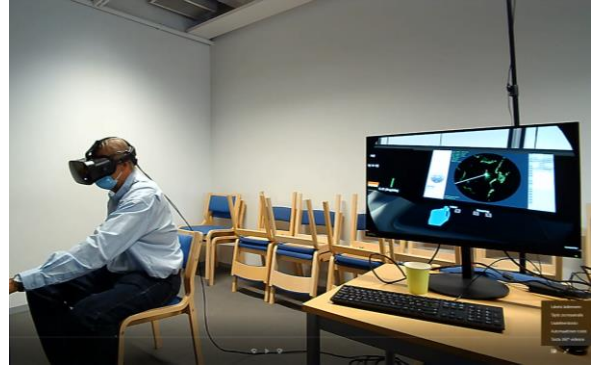
Figure 5: An experienced seafarer testing the bridge controls and ship behavior during the system development.
