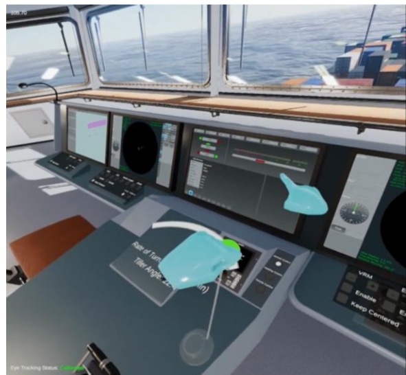
Figure 3: Tiller use implements a larger hand movement than usual and a virtually produced information about the rate of turn and angle.
