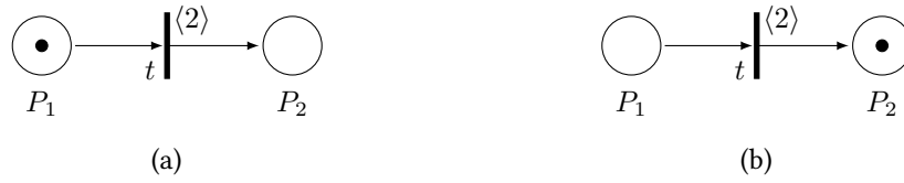
Figure 3: TdPN of a sending process: (a) shows the initial marking before sending, and (b) shows the marking after sending. P_1 represents the node's internal state of 'before sending' and P_2 the state of 'done sending'. The transition t , which represents the sending, takes the time 2.
