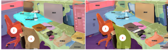
Figure 2: Instance labels obtained from panoptic segmentation. chair_1 (resp. chair_2) of the left image is the same instance as chair_4 (resp. chair_3) in the right image.
