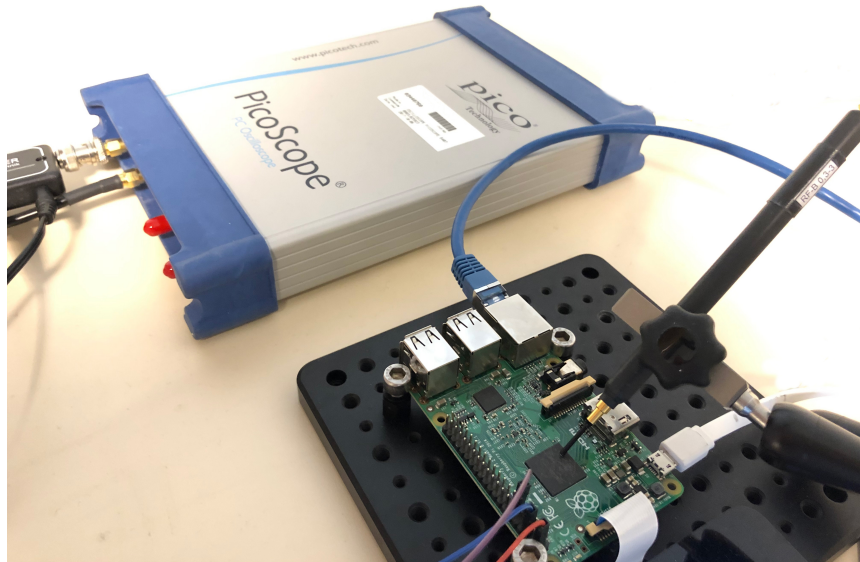
Figure 1: Probe setup consists of a H-Field probe placed 45 degree above the system processor.
